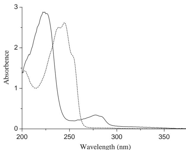
Fig. 3. Ultraviolet–visible spectra of IVM (---) and zein (—) in 66.7% ethanol. The coefficients of light extinction of IVM and zein at 245 nm are 351.5 and 7.1, respectively.
