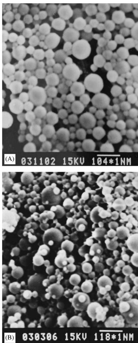
Fig. 1. Scanning electron micrographs of IVM-loaded zein microspheres prepared by the phase separation method. (A) Before lyophilization, the scale bar is 1.04  $\mu\text{m}$ ; (B) after lyophilization, the scale bar is 1.18  $\mu\text{m}$ .
