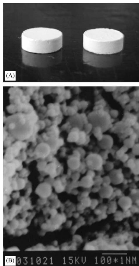
Fig. 2. Outward of the tabletted microspheres (A) and scanning electron micrograph of the internal structure (B) after compressing and shaping in wet box at 37°C for 3 days, the scale bar is 1  $\mu\text{m}$ .
